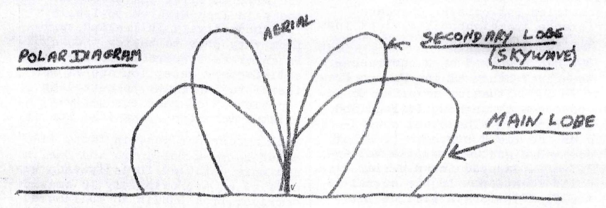
This lobe causes a strong skywave to be radiated to the ionosphere where it is reflected and at a short distance from the transmitter meets the ground wave giving rise to fading. So if the onset of fading is to be kept at a maximum distance from the transmitter the height of the mast must be about half a wavelength.
